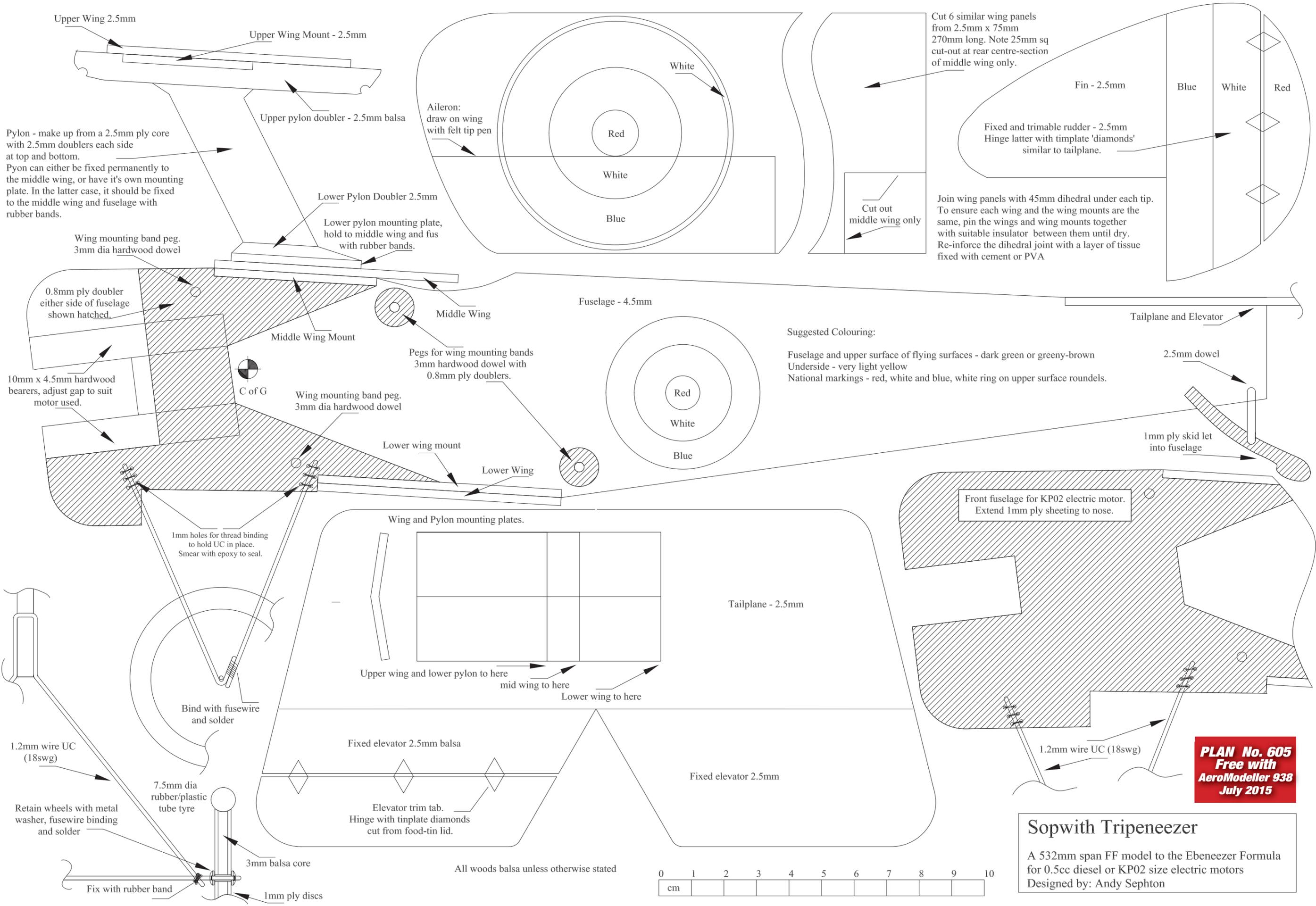
Pylon - make up from a 2.5mm ply core with 2.5mm doublers each side at top and bottom. Pylon can either be fixed permanently to the middle wing, or have it's own mounting plate. In the latter case, it should be fixed to the middle wing and fuselage with rubber bands.
